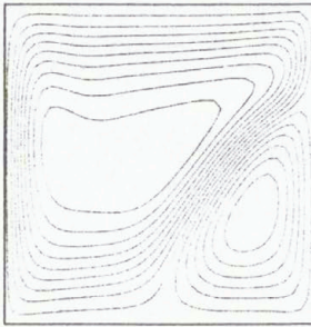
Numerical simulation adiabatic walls. Stream function (left), velocity field (right)
