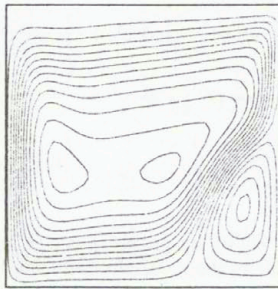
Numerical simulation conducting walls. Stream function (left), velocity field (right)
