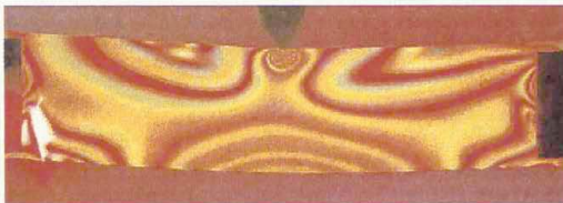
Fig.4 : Photographic visualization of isochroms at shock contact on rectangular plate.
